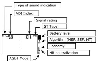
VDI means Visual Discrimination Indication. VDI Index This is a so-called electrical conductivity indication of the object.
